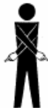
Land Arms crossed in front of body and pointing downward with back to wind.
