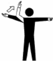
Move Right Left arm horizontal, right arm sweeps upward to position over head.
