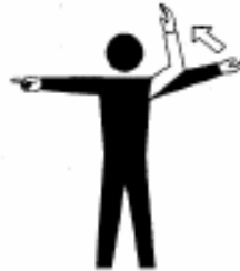
Move Left Right arm horizontal, left arm sweeps upward to position over head.
